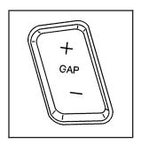
Use the GAP button on the steering wheel to adjust the follow distance.
